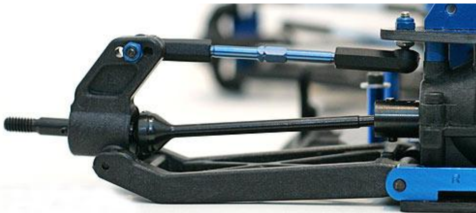
Fig. 7. Electric 4wd chassis CVD drive used rear and front.
