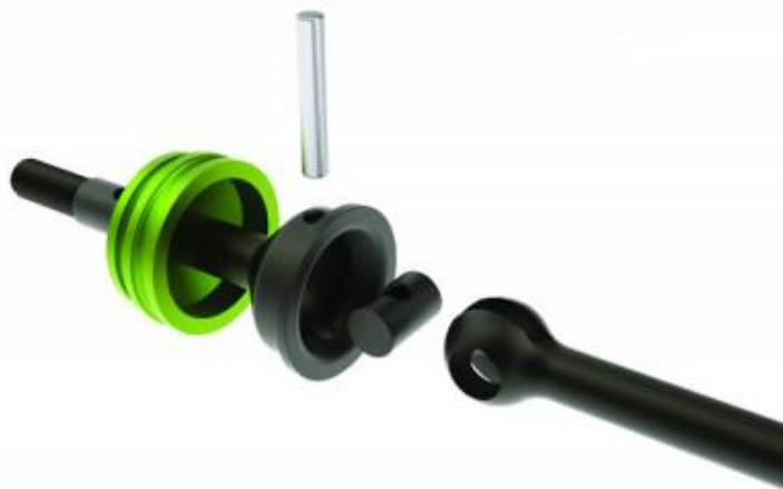
Fig. 3. CVD Transmission used in off-road chassis
